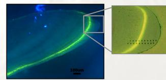
Sectioned otolith showing OTC mark (=expt start) and 20µm spots made by SIMS for  $\delta^{18}O$  analyses. Spot sizes for trace metals were 8µm on SIMS and 35µm on LA-HR-ICPMS
