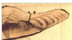
Left: Photograph of the sectioned otolith shows the pits left by the LA-ICPMS analyses (see Methods).
